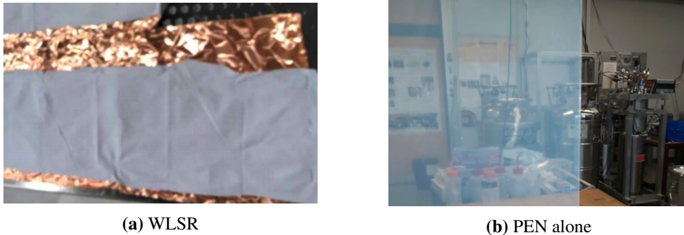
Figure 4.2: (a) WLSR witness sample from the LEGEND-200 in-situ TPB deposition at LNGS. (b) PEN sample without reflector and without sanding (milky plastic in the photo).
