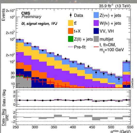
A combined signal+background fit is performed on the MET distributions in the different channels. Systematics due to resolution and efficiency of the detector, theory assumptions, reconstructions of the objects, are also taken into account.
