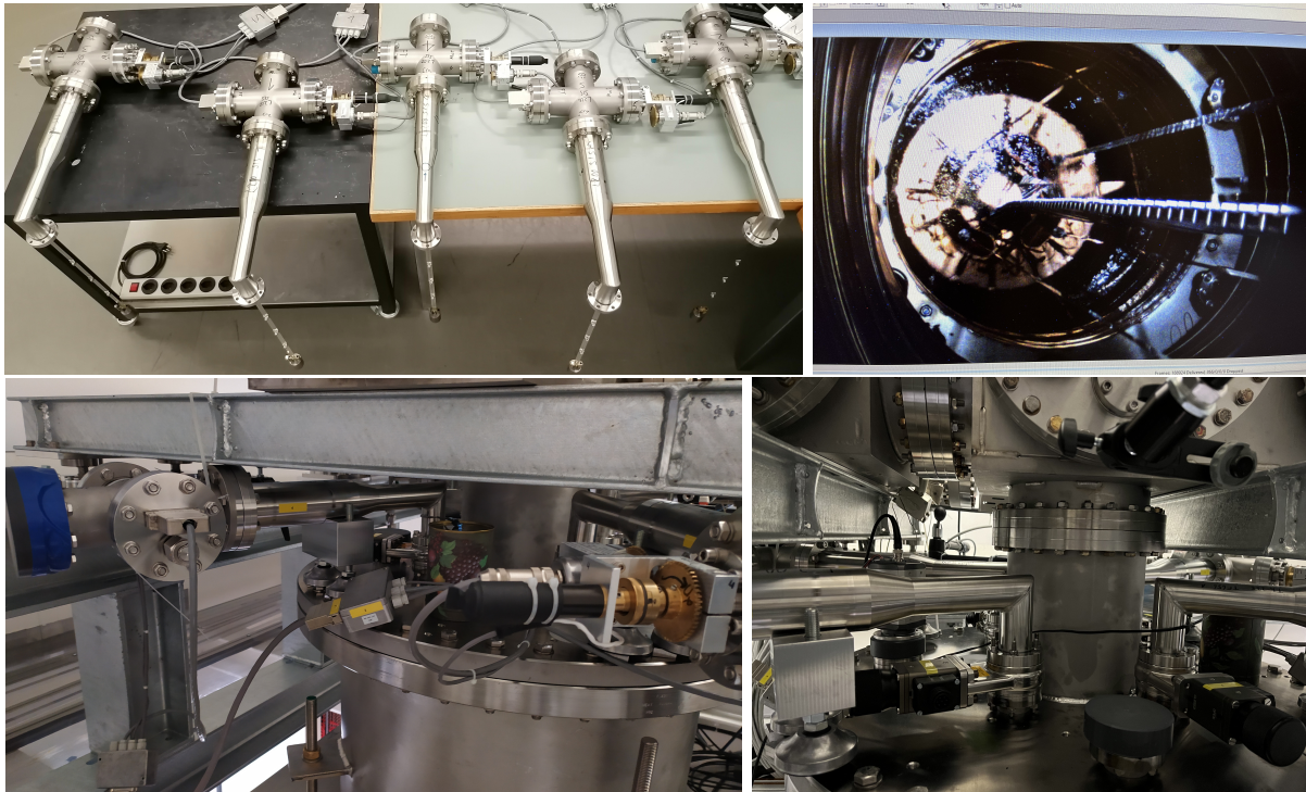
Figure 3.4: Top left: picture of the five L-200 calibration source insertion system after assembly at UZH. Top right: view into the L-200 cryostat when the sources are lowered to the detector array. The photo was taken with a camera installed above the cryostat. Bottom: pictures of the SIS mounted on top of the lock system at LNGS.
