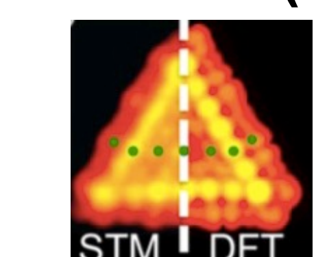
Figure 8: STM image and DFT model of a MoS_2 cluster on Au(111) [5]
