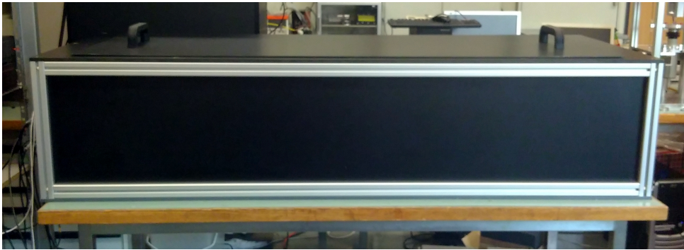
Figure 2.12: The dark box used in the lab to shield the test setup from light.
