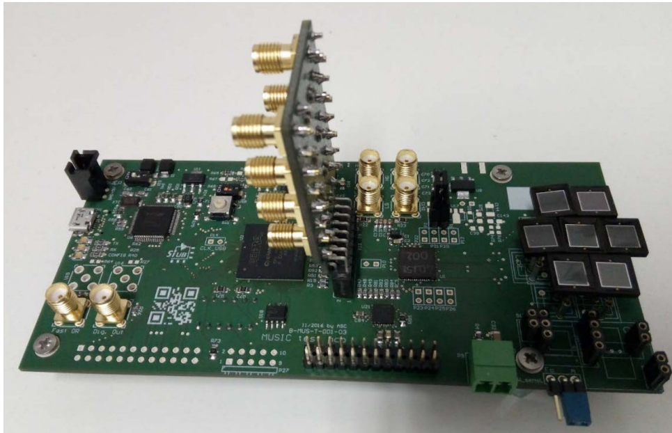
Figure 2.8: The frontside of the MUSIC-board with SMA board for individual readout and 7 Hamamatsu HPK-S13360-6050CS connected on right. [28]
