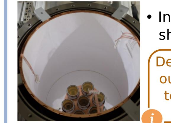
Installation of wavelengthshifting Tetratex reflector foils
