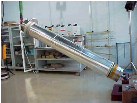
Figure 15.3: A completed detector cylinder is prepared for removal from the mandril.
