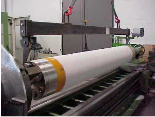
Figure 15.1: A Rohacell cylinder on its mandril is being prepared for polishing.
