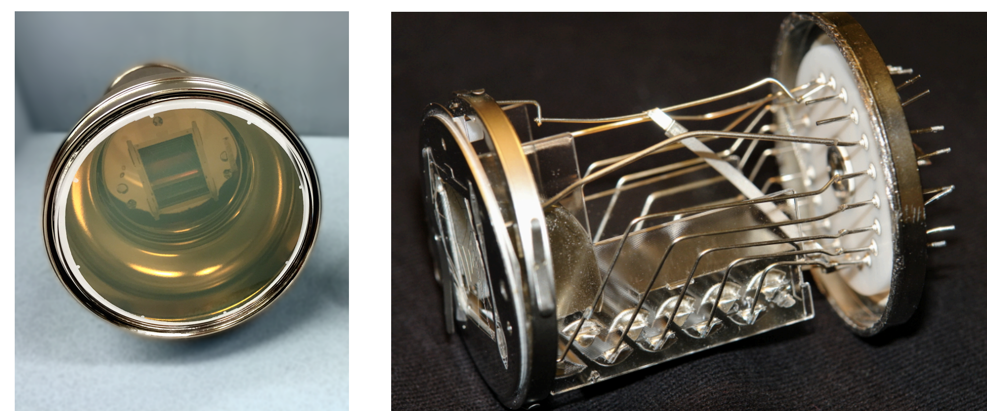
R11410-21 (left) and its dynodes (right)
