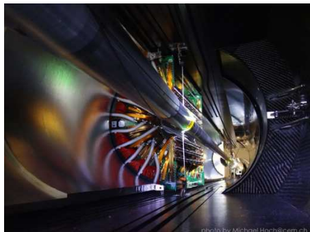
FIG. 11.10 – One half of the barrel pixel detector after re-installation in CMS.
