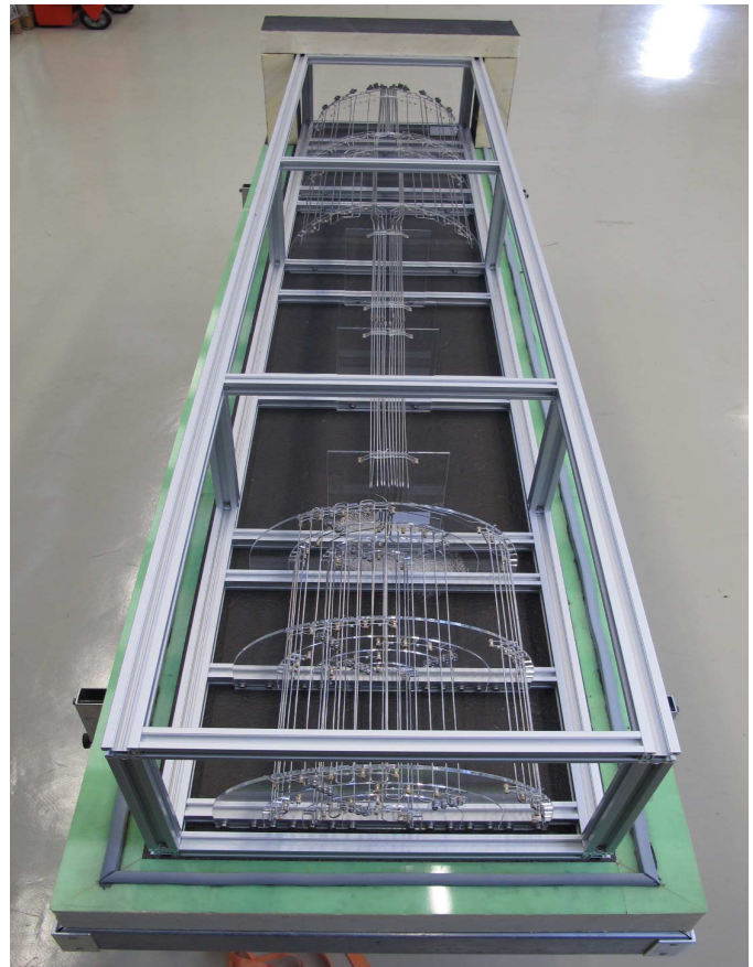
FIG. 11.14 – One of the two half-barrel prototypes of the phase 1 pixel upgrade cooling system.
