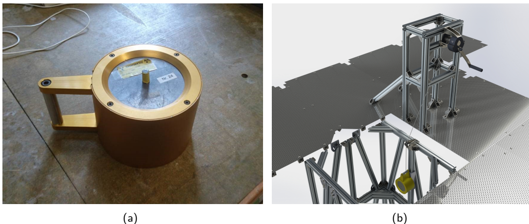
Figure 43: (a): Picture of the collimator used for this project. (b): Render of the top part of the collimation setup designed with SolidWorks. In the proposed but not yet built setup, the Xenoscope cryostat would sit in front of the collimator and was hidden in the render for a better view.
