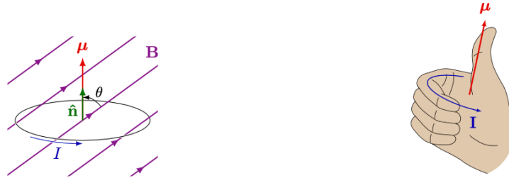
(a) Magnetic moment of a current loop in a uniform magnetic field.
