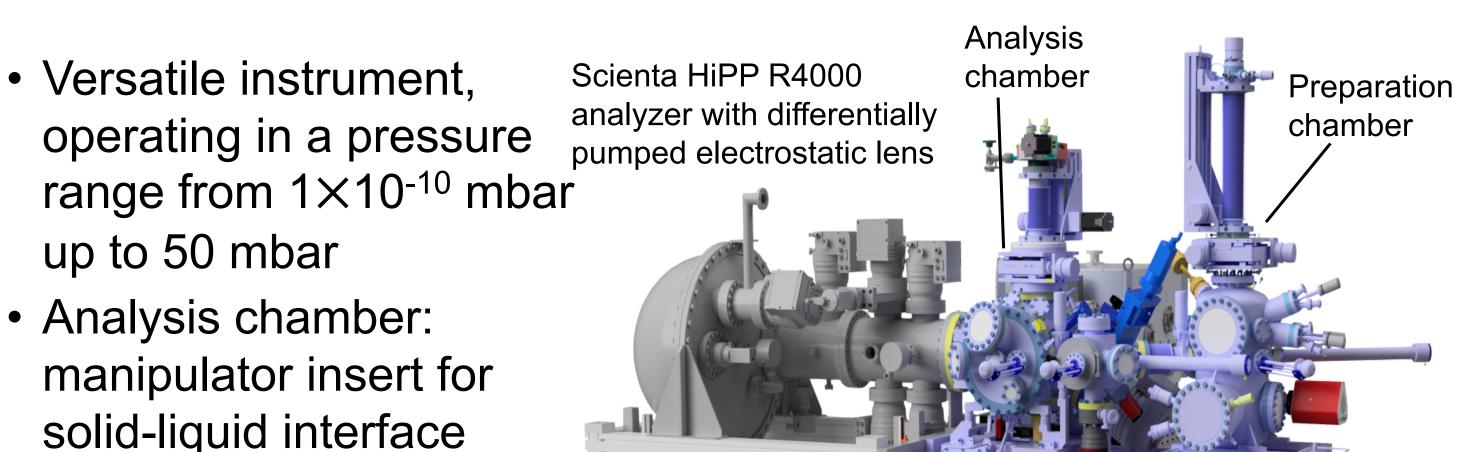
With tender X-rays (here 4 keV) and electrolyte layer thickness between 20-30 nm, we can probe the solid-liquid interface for the first time using single crystalline surface
